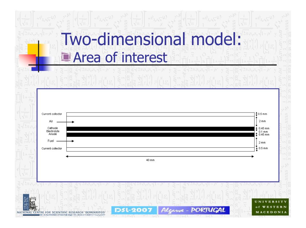
**Two-dimensional model:** Differential equations  $\nabla \underline{u} = -\nabla p + \mu \nabla^2 \underline{u}$ Flow  $\nabla \cdot \left[ \left( \rho c_p T \right) \underline{u} \right] = \dot{Q} + \nabla \cdot a \nabla \left( \rho c_p T \right)$ Heat  $\underline{u} \cdot \nabla C_i - \nabla \cdot \left( D_{i,mix} \nabla C_i \right) = 0$ Mass  $\left(\frac{a_a F}{RT}\eta\right) - \exp\left(-\frac{a_c F}{RT}\eta\right)$ Charge exp
