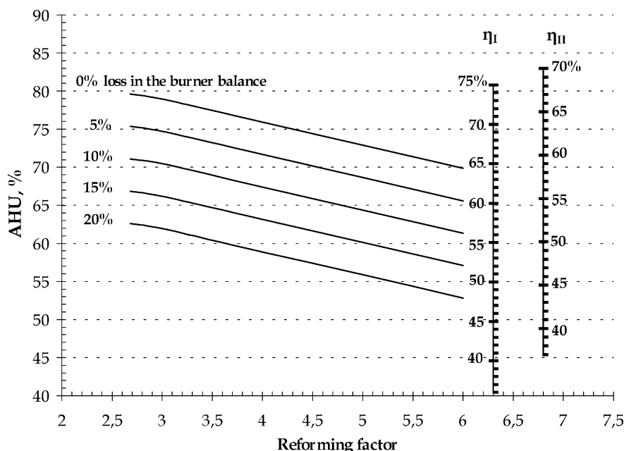
Fig. 7. Nomograph of the first and second law efficiencies for various reforming factors and burner balances ( \varepsilon = \varepsilon_{max} , optimum \Delta T_{sofc} , T_{sofc,out} = 1200 K).
