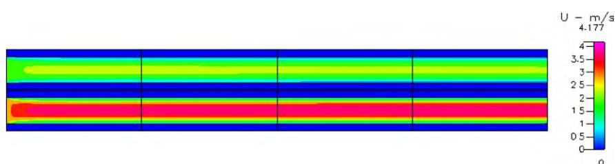
Fig. 6 – Velocity profile for non-isothermal conditions.
