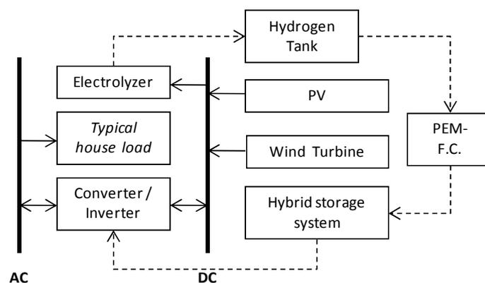
**Figure 6.9** The components of the hybrid system with hydrogen technology.
