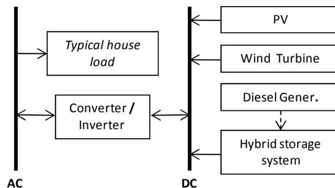
**Figure 6.8** The components of the hybrid system with a diesel generator.
