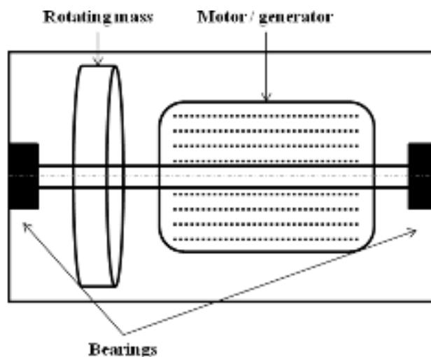
**Figure 6.2** Design of a typical FESS.
