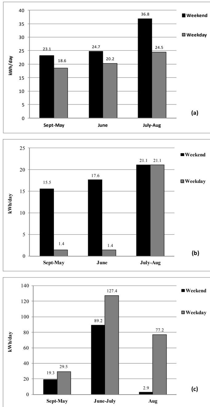
**Figure 3.9** Average load requirements per day for a typical house (a), a typical country house (b), and a typical small enterprise (c).
