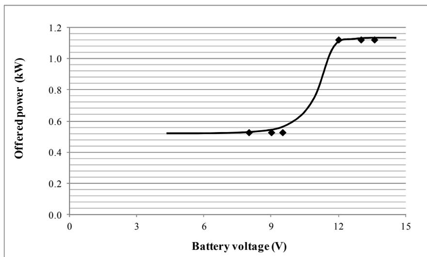
**Figure 5.5** Energy offered by the battery bank as a function of voltage.
