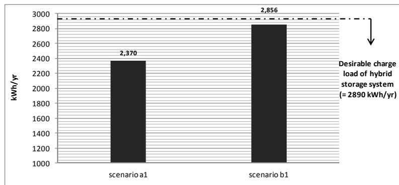
**Figure 6.12** The desired annual electrical energy of the hybrid storage system using a flywheel with a Hoppecke 3 kAh battery.
