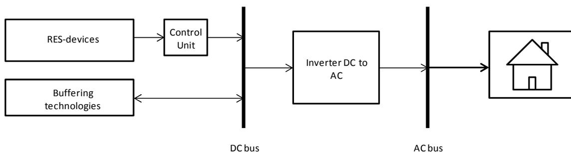
**Figure 2.4** A typical off-grid RES-based hybrid system.
