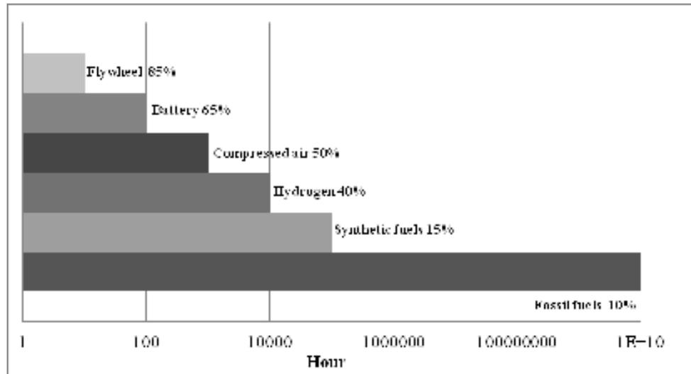
**Figure 6.1** Comparison of different technologies in terms of efficiency as a function of time (Ledjeff, 1990).
