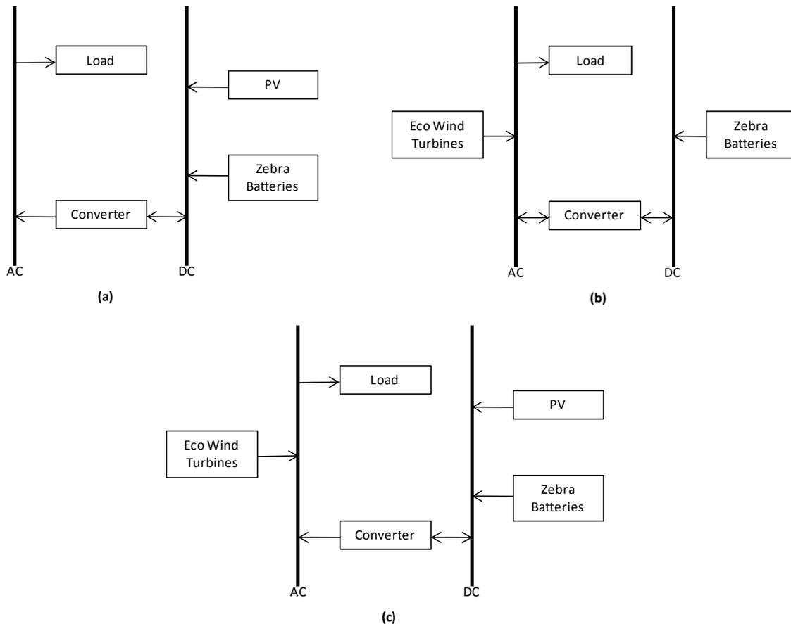
**Figure 3.8** The components for a single photovoltaic (a), a single wind turbine (b), and a hybrid photovoltaic-wind (c) system.
