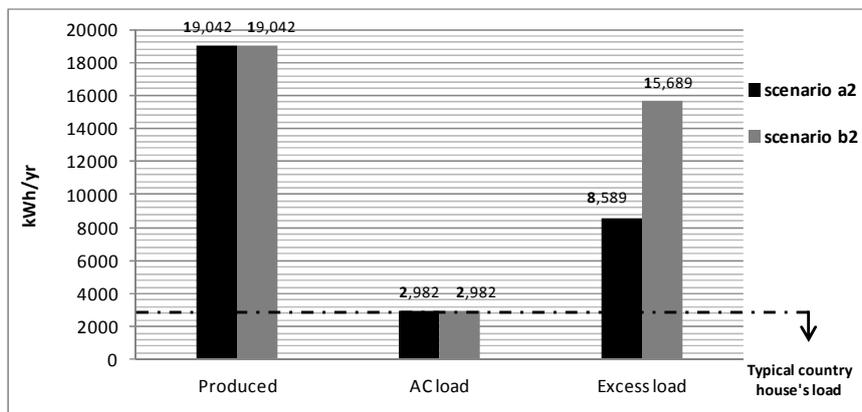
**Figure 6.11** Produced, AC-primary and excess load for each system (load = typical country house).
