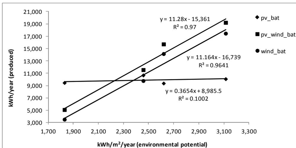
**Figure 3.10** The produced electricity as a function of environmental potential.
