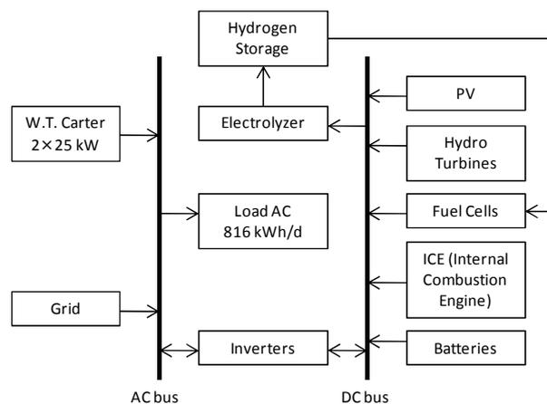
**Figure 3.1** Schematic view of the RES based system at West Beacon Farm, Leicestershire, UK.
