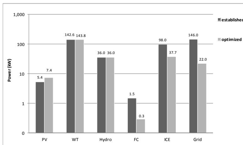
**Figure 3.2** Electricity production per RES device of the West Beacon Farm system to cover the peak electricity demands (established) and a more realistic load (optimized).
