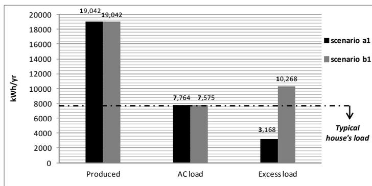
**Figure 6.10** Produced, AC-primary and excess load for each system (load = typical house).
