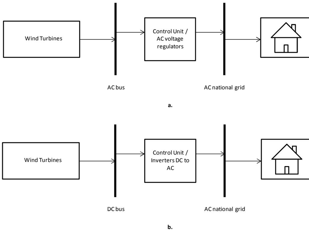
**Figure 2.3** (a) Connection of an AC load wind farm to the national grid, (b) Connection of a DC load wind farm to the national grid.
