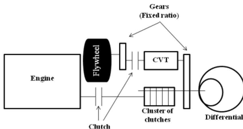
**Figure 6.3** The Kinetic Energy Recovery System (Tripathy, 1992, 1994).
