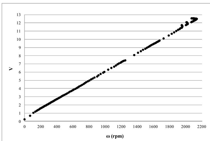
**Figure 6.17** The operational curve of the electric motor with no load.
