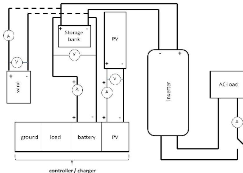
**Figure 5.1** Schematic circuit diagram of the laboratory-scale system.
